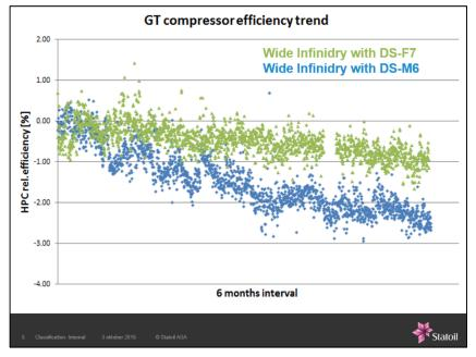
As part of the upgrade process from Wide IFD DS-M6 to Wide IFD DS-F7, Statoil run extensive side-by-side benchmarking on the Sleipner field in the North Sea during 2015 and 2016 for consecutive real-life testing and verification, with the following performance result, as reported by Statoil.
